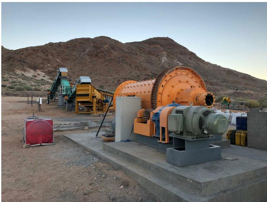
**Aukum Plant commercial scale rod mill, screeners and conveyance systems**
