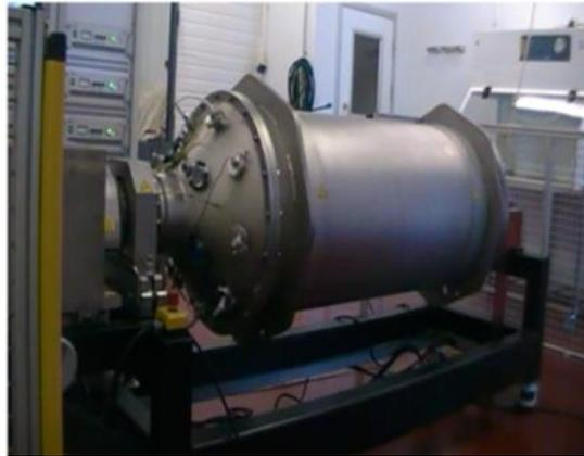
Triple chamber reactor – 500 tpa capacity
