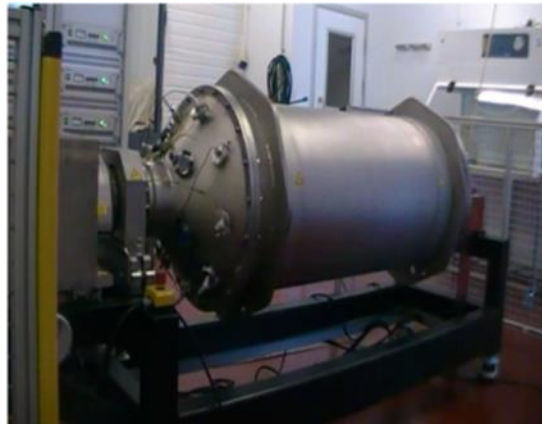
Triple chamber reactor – 500 tpa capacity
